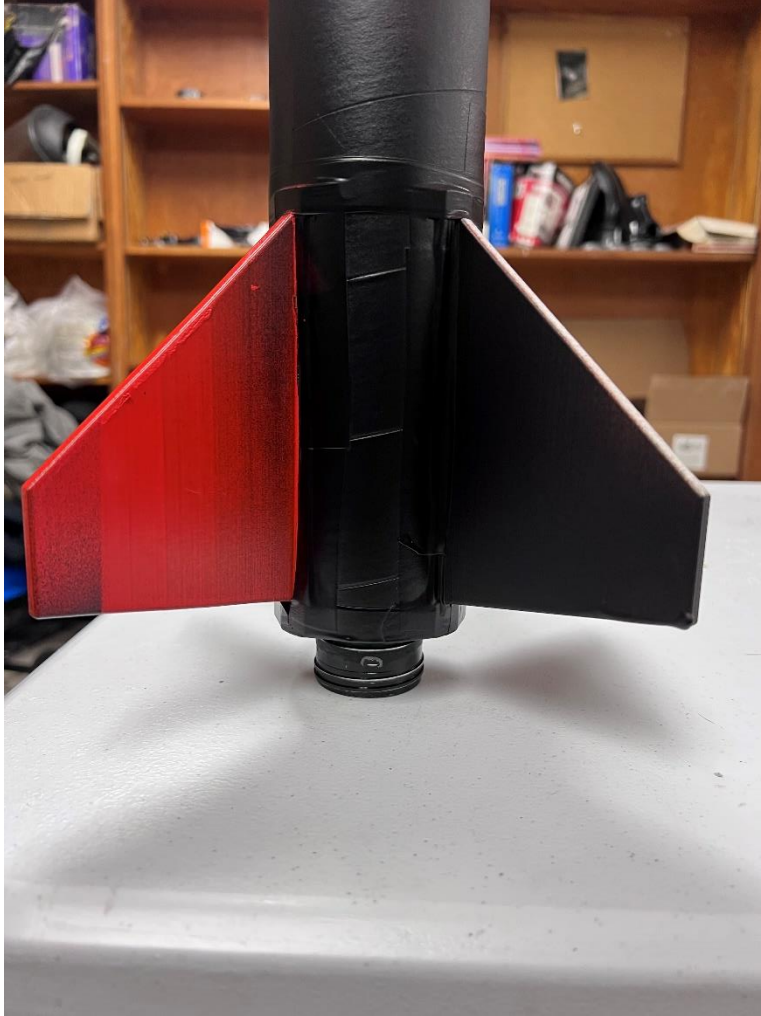
Figure 3-45. Subscale Fins Installed
